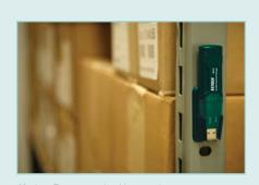
Monitors Temperature level in a warehouse or storage room.
